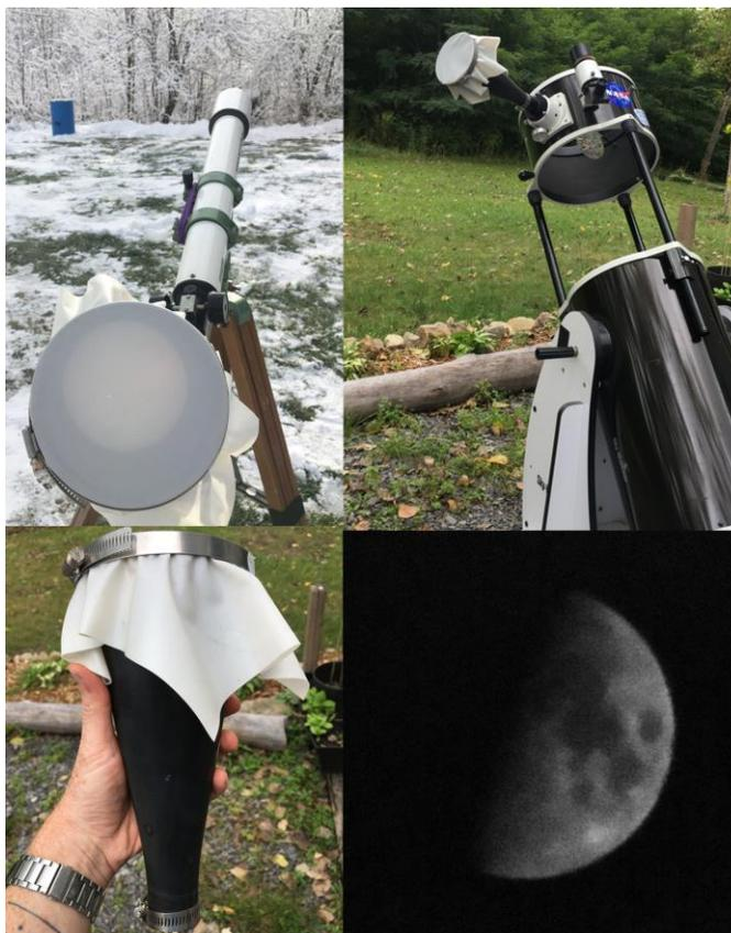
Caption: Sun Funnels in action! Starting clockwise from the bottom left, a standalone Sun Funnel; attached to a small refractor to observe the transit of Mercury in 2019; attached to a large telescope in preparation for evening lunar observing; projection of the Moon onto a funnel from a medium-size scope (5 inches).
