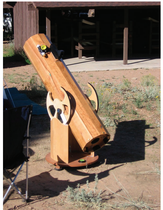
Image Caption: Telescopes of interesting design/configuration always show-up at RTMC, including this 11-inch refractor on a portable Volvo Mount and this homemade 8-inch wooden Dobsonian. Image Credit: Alan Gorski
