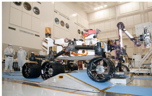
Caption: The Mars Science Lander being assembled in a clean room at the NASA Jet Propulsion Laboratory.
