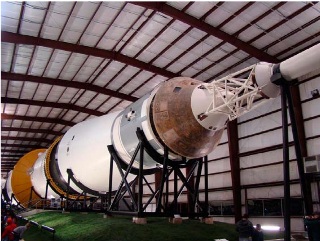
Caption: The massive Saturn V is nestled inside of its new climate controlled home at Rocket Park, Houston. The Saturn V is 363 feet in length, and the five F-1 engines of the first stage generated about 7.5 million pounds of thrust at launch. At launch, the vehicle weighed about 6.7 million pounds, of which over 90% was fuel. The first stage, powered by RP-1 Kerosene and liquid oxygen, operated for about 2 minutes 40 seconds, carrying the vehicle to an altitude of ~42 miles and a speed of ~5300 mph. The second and third stages consisted of five and one J-2 engine(s), respectively, and they were powered by liquid hydrogen and liquid oxygen. The J-2 was the first restartable rocket engine. The third stage J-2 provided the remaining power necessary to put the vehicle in Earth orbit. It was later fired for about 6 minutes to send the Command/Service Module and the LM to the Moon. For more information see Wikipedia. Photo Credit: Karen Harris
