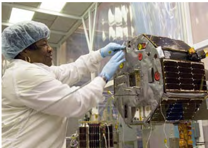
Helen Johnson, a spacecraft technician at NASA's Goddard Space Flight Center, works on one of the three tiny Space Technology 5 spacecraft in preparation for its technology validation mission.
