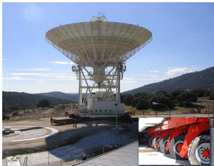
Giant Deep Space Network antenna in Madrid is moved using four 12-axle, 24-wheel crawlers.
