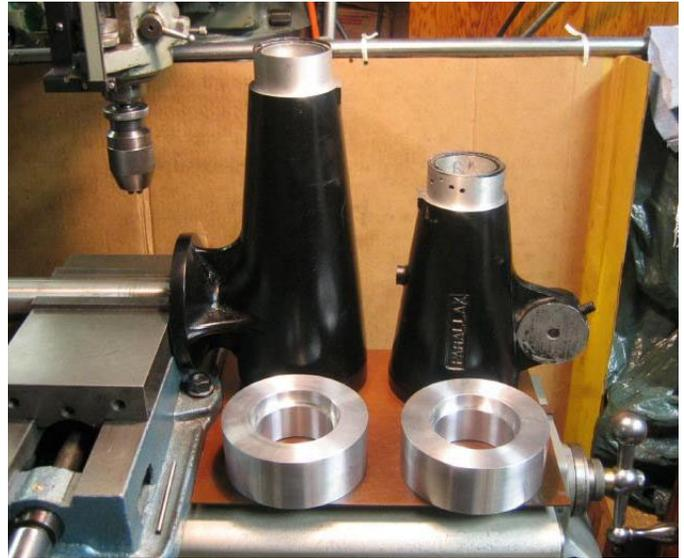
The RA and Dec shafts of the Marling scope. The silvery metal pieces are the newly machined parts.
