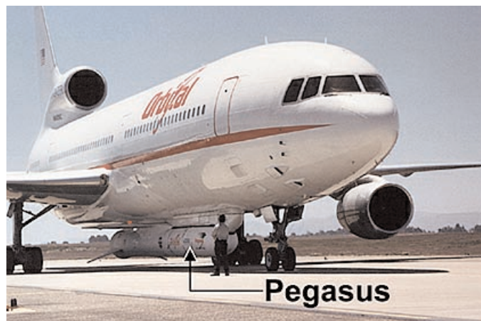
L-1011 "Stargazer" takes off to carry Pegasus rocket on the first 39,000 feet of its climb to deliver a spacecraft to orbit.
