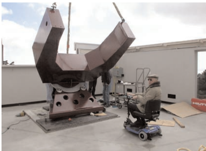
Nellie's fork arm. Merrill Martin, the major donor for the construction of Nellie, is on the right.
