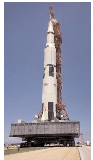
The Saturn V and Mobile Launch Platform are carried to the launch pad on the Crawler Transporter. Notice the tiny humans below the platform.
