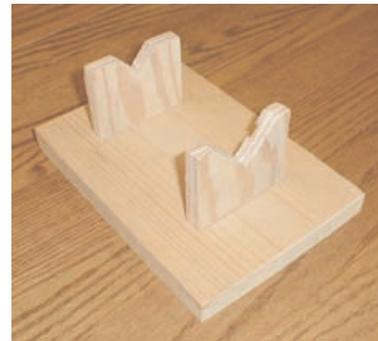
one end, and drill a  $3/32$ " pilot hole. All you need is one pilot hole per support to get you started; the deck screws can work their way into the support on the other hole without splitting the wood if centered properly. Insert one of the screws through the base plate and into the pilot hole. Screwing it snug, but not tight, swing the support into position and insert and tighten the second screw. Do this on the other end and you are done!
